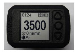
While in Climb Mode the settings of the device can be accessed and changed.
