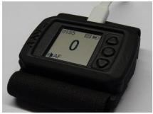
The device can as well be charged also while placed in the wrist mount as the external housing allows the access to the USB connector, from both sides.
