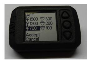
The canopy alarms sound prior to the configured altitude and stop when reaching it.
