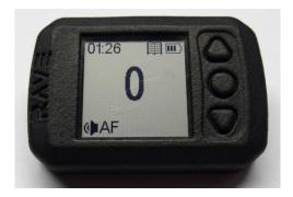
Pressing the "Down" button switches the display to Free Fall mode.
