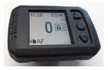
Your RAVE altimeter comes with a set of default parameters, please configure it before using it for skydiving activities according to your needs: language, alarm intensity, altitude trigger levels, metric vs. imperial measurement units, etc. Refer to the chapter 4. Menu for details.
