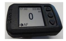
Pressing the "Down" button switches the display to Free Fall mode.
