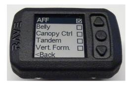
The freefall alarms sound when the altitude is reached. The 3<sup>rd</sup> freefall alarm is a special emergency alarm: it will sound continuously if the descent speed is high (freefall speed) at the configured altitude or below, i.e. beyond the safety zone.
